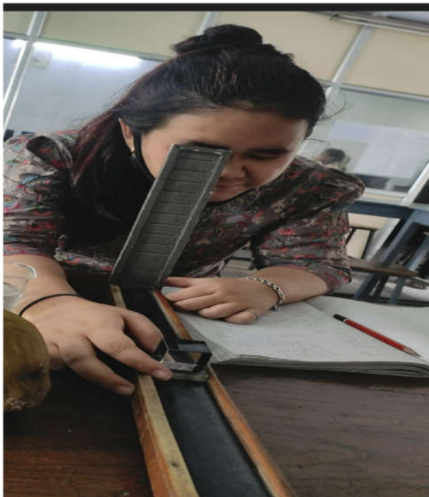
figure 1 a Measurement of total internal reflection using Pulfrich Refractometer
