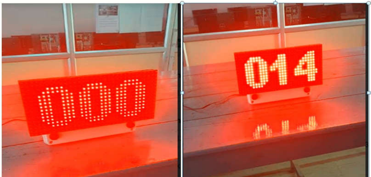
Figure 2 a Bi Directional Counter showing the Number of students in the lab before and after the class
