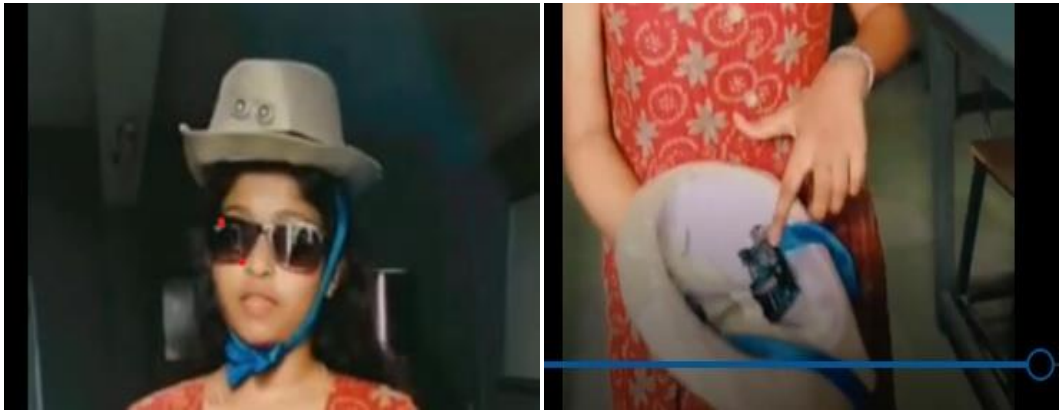
Figure 1b & 1c The physical picture of the assistive hat and consisting of: Ultrasonic sensor HC-SR04, reset button, Arduino Nano board, vibrators and buzzer.
