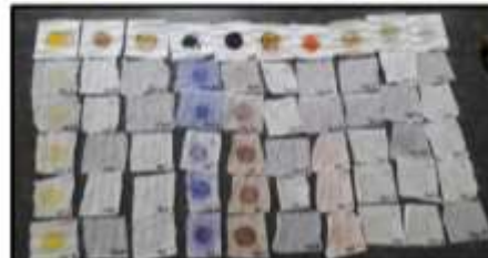
Fig. 4. Stained cloths, treated with detergents having unknown composition, dried and segregated.
